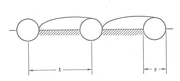
Figure 5. Cavitation model. Ellipsoidal cavity bubbles trail behind round grains. The grains are small enough that the ambient pressure several grain diameters above them is the surface pressure  $p_s$ .
